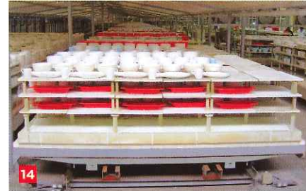
7 Venezuela: Kiln cars 6500x4300 mm 8 Mexico: Construction of kiln cars 6800x4500 mm 9 Algeria: Tunnel kiln walls and suspended roof under going construction 10 11 12 France: New generation energy saving kiln car system for H and U cassettes 13 14 15 16 Portugal: LIZCORITE batts, supports and kiln car perimeter blocks
