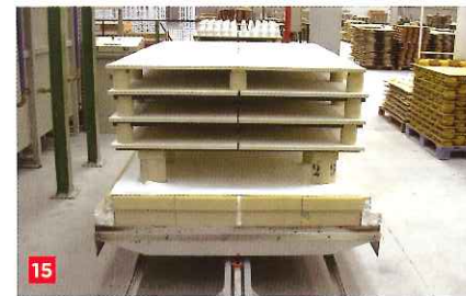
7 Venezuela: Kiln cars 6500x4300 mm 8 Mexico: Construction of kiln cars 6800x4500 mm 9 Algeria: Tunnel kiln walls and suspended roof under going construction 10 11 12 France: New generation energy saving kiln car system for H and U cassettes 13 14 15 16 Portugal: LIZCORITE batts, supports and kiln car perimeter blocks
