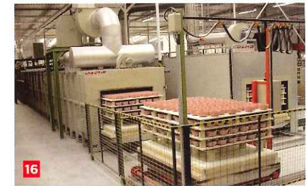
7 Venezuela: Kiln cars 6500x4300 mm 8 Mexico: Construction of kiln cars 6800x4500 mm 9 Algeria: Tunnel kiln walls and suspended roof under going construction 10 11 12 France: New generation energy saving kiln car system for H and U cassettes 13 14 15 16 Portugal: LIZCORITE batts, supports and kiln car perimeter blocks
