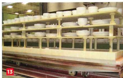
7 Venezuela: Kiln cars 6500x4300 mm 8 Mexico: Construction of kiln cars 6800x4500 mm 9 Algeria: Tunnel kiln walls and suspended roof under going construction 10 11 12 France: New generation energy saving kiln car system for H and U cassettes 13 14 15 16 Portugal: LIZCORITE batts, supports and kiln car perimeter blocks
